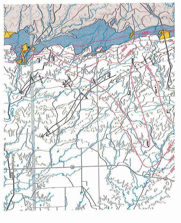
Potentiometric surface of Madison is not directly inferable from current mapping data. Possibly 3000'-3100' (400'-500') below GL
